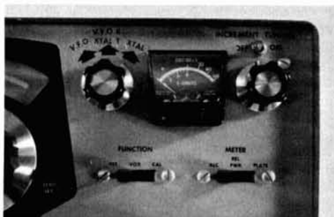
Front panel of the modified HW-100 showing the crystal/vfo control switch.
